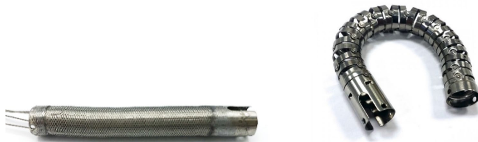
Figure 1. Example of a bending section in a typical state of the art endoscope—with welded mesh and mounted bowden wires (left) and the pure inner bending section (right, device class OD 10 mm), Source Endoscopeparts.com ® .
