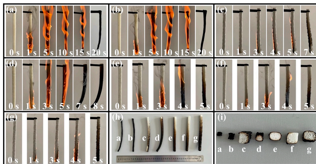
Figure 6. Digital photographs of VFT for samples of (a) neat RPUF; (b) SA/RPUF; (c) 8EG/SA/RPUF; (d) 8APP/SA/RPUF; (e) 2EG/6APP/SA/RPUF; (f) 4EG/4APP/SA/RPUF; (g) 6EG/2APP/SA/RPUF; (h) the external appearance; (i) the cross-section of the samples after VFT.
