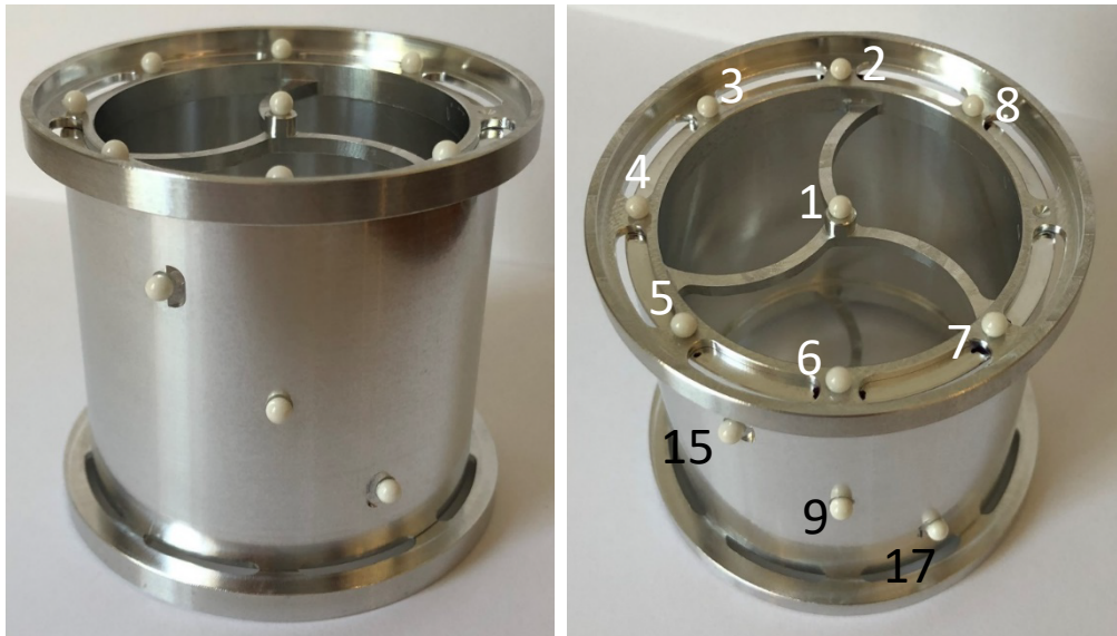
Fig. 6. Physical embodiment of the reference object in Fig. 5 with 18 spheres distributed among three planes. Spheres 1–8 are arranged on a circle with a nominal diameter of 50 mm, while the spheres in the top and bottom planes are nominally 50 mm apart.
