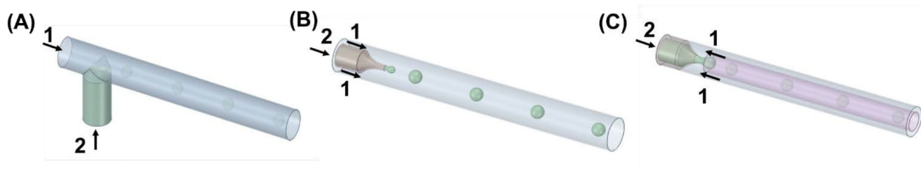
Figure 5. Microfluidic geometries are used to generate droplets. (A) T-junction, (B) co-flow, (C) flow-focusing. (1: continuous phase, 2: dispersed phase). Reproduced from Zhang et al. [75], with permission from Elsevier.
