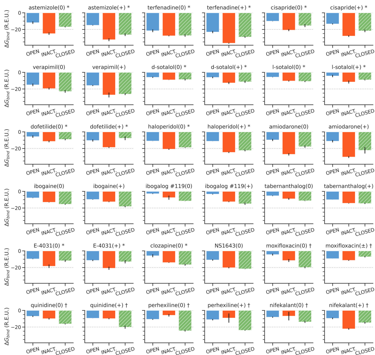
Figure S11. GALigandDock drug docking results to different hERG channel models. Each bar plot represents the estimated free energy of binding in Rosetta energy units (R.E.U.) for the named drug to the open-, inactivated, and closed-state hERG channel models. Lower values mean more favorable binding. 25,000 docking poses were generated for each drug/channel model pairing. The top 50 poses were clustered, and the plotted energy represents the average free energy of the top cluster along with the standard deviation. The first suffixes (0), (+), and (±) indicate whether the drug is in the neutral, cationic, or zwitterionic form, respectively. The second suffixes * and † indicate validation from experimental studies (Alexandrou et al., 2006; Numaguchi et al., 2000; Perrin et al., 2008; Wang et al., 1997) showing whether the drug prefers binding to hERG inactivated state (*) or does not (†), respectively.
