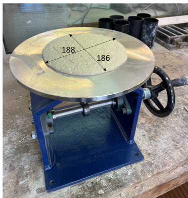
Figure 5. Fresh mortar mix consistency test for geopolymer mortar (measurements in mm).
