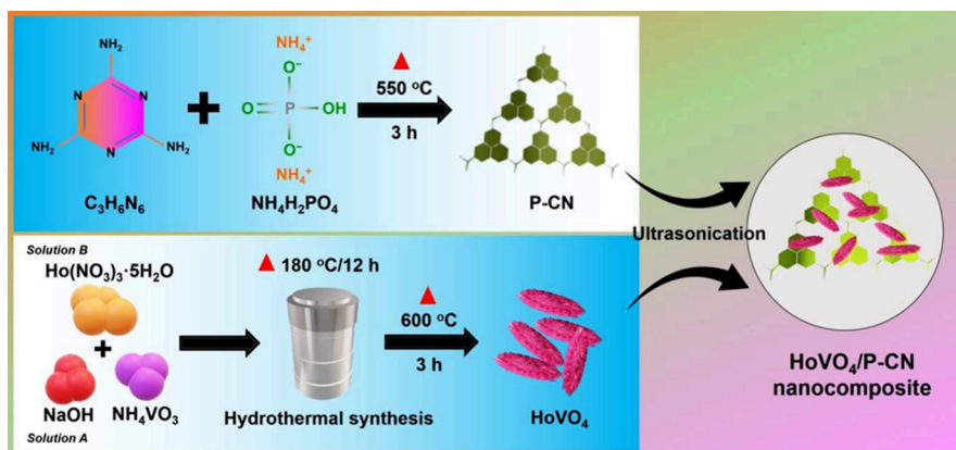
Scheme 1. Schematic Diagram for the Preparation of the HoVO 4 /P-CN Nanocomposite
