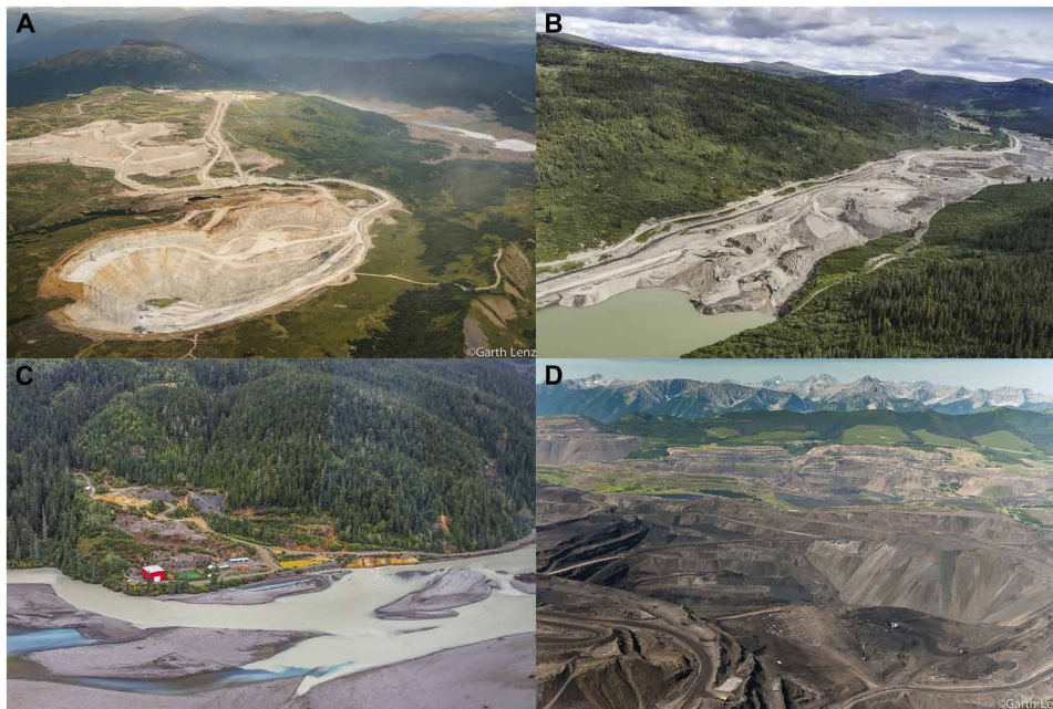
Fig. 2. Representative mining operations in northwestern North America. (A) Open-pit operations with a wet tailings impoundment facility beginning to take shape in the background (Red Chris Mine, BC; Garth Lenz). (B) Open-pit placer operations with a pit lake used for recirculating sluicing water (Atlin, BC; Jackie Caldwell). (C) Legacy underground operations adjacent to a glacial river (Tulsequah Chief Mine, BC; Christopher Sergeant). (D) Mountaintop removal coal mining (Elk Valley, BC; Garth Lenz).
