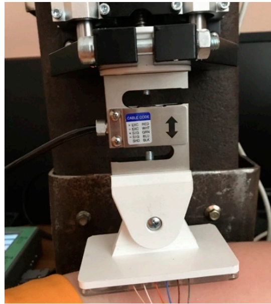
Figure 7. Design of attachment of the strain gauge and electrode system in the laboratory facilities.
