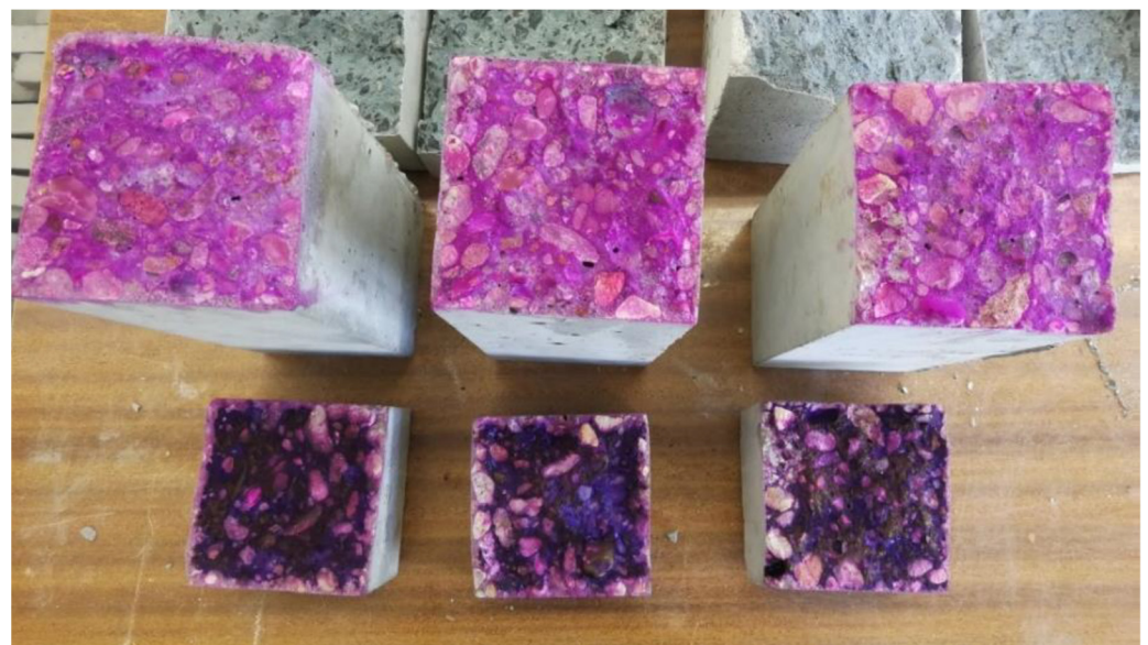
Figure 4. Concrete specimens are used to test the depth of carbonation with the indicator recommended in the EN 13295:2004 standard [35], i.e., phenolphthalein (indicating pH \sim 8.5 )—upper row and thymolphthalein (indicating pH \sim 9.5 )—lower row; the uncolored area at the fracture edges indicates a carbonated area.
