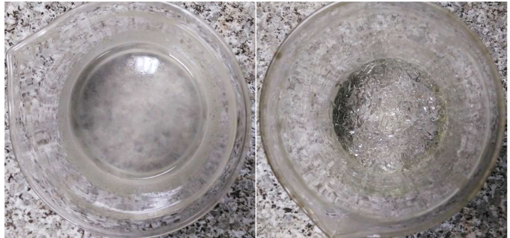
Figure 6. Macro-observations of SAP particles saturated with a solution of mixing water and a superplasticizer admixture (left) and saturated with mixing water with no admixture (right) show the synergistic effect between SAP and superplasticizer.
