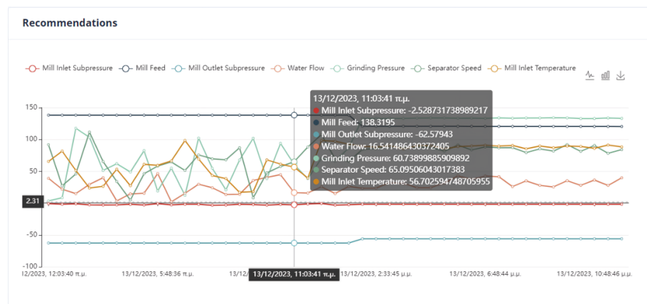
Figure 23. Comparison between actual and recommended values of parameters in the mill in the first optimization strategy.
