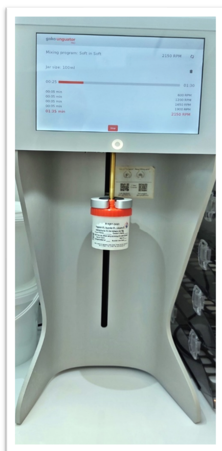
Figure 2. Electronic mortar and pestle: A modern tool essential for compounding pharmacies, this enables mixing preparations directly in the dispensing container. It is innovatively designed to enhance pharmaceutical compounding, produce refined preparations, and reduce nonproductive time (Courtesy pharmacist Eyal Zur).
