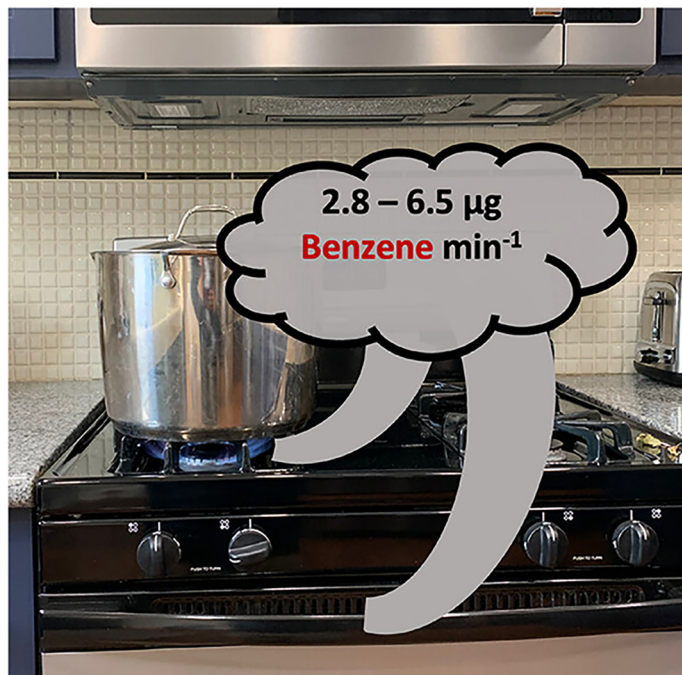
Incomplete combustion of natural gas during normal operation of home appliances generates measurable levels of methane, carbon dioxide, and nitrous oxides, left, and benzene, right. Images: Lebel et al. (2022), left 5 ; Kashtan et al. (2023), right 10 ; both CC-BY-NC-ND 4.0. [ https://creativecommons.org/licenses/by-nc-nd/4.0/ ].
