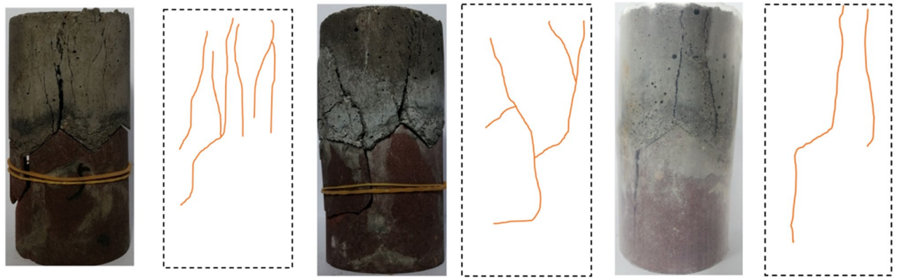
Figure 5. Failure crack diagram of sandstone–concrete combined body.
