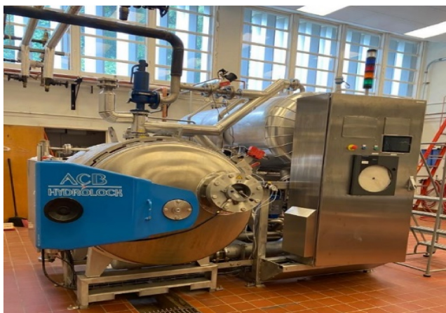
FIGURE 5 Retort ACB Hydrolock (Photo courtesy of Cryovac® Flavor Mark® Retort Laboratory, Clemson University, SC).
