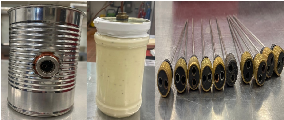
FIGURE 6 Assemble thermocouples in glass jars and metal cans (Photo courtesy of Cryovac® Flavor Mark® Retort Laboratory, Clemson University, SC).
