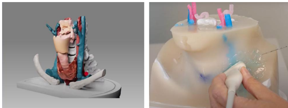
Figure 2 The ad-hoc 3D model designed for operators' training. This model consists of 3D printed anatomical structures (on the left) plunged in an agar-based gel (on the right) which produces the same echogenicity as the human body
