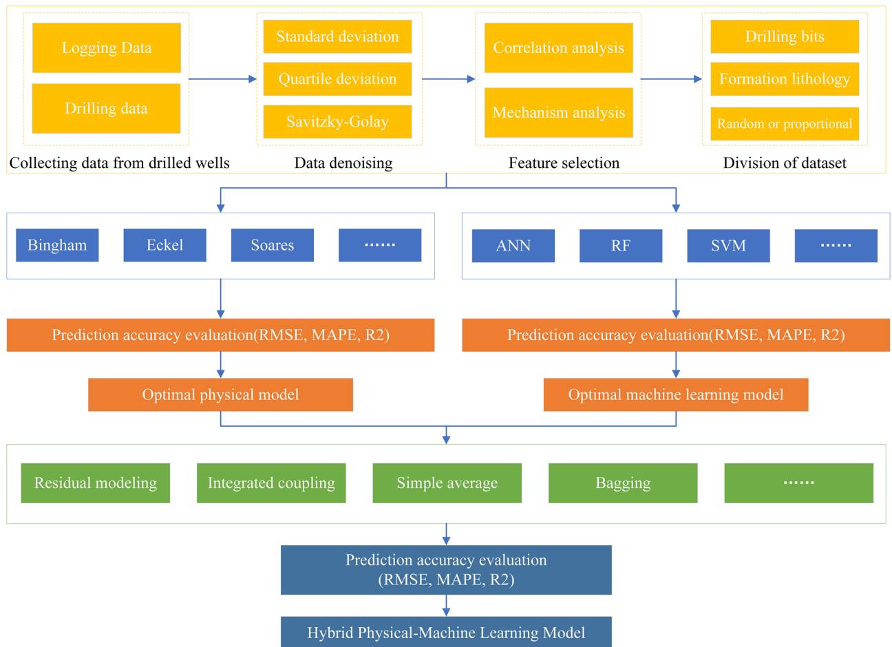
Figure 1. Procedure of the hybrid ROP modeling.
