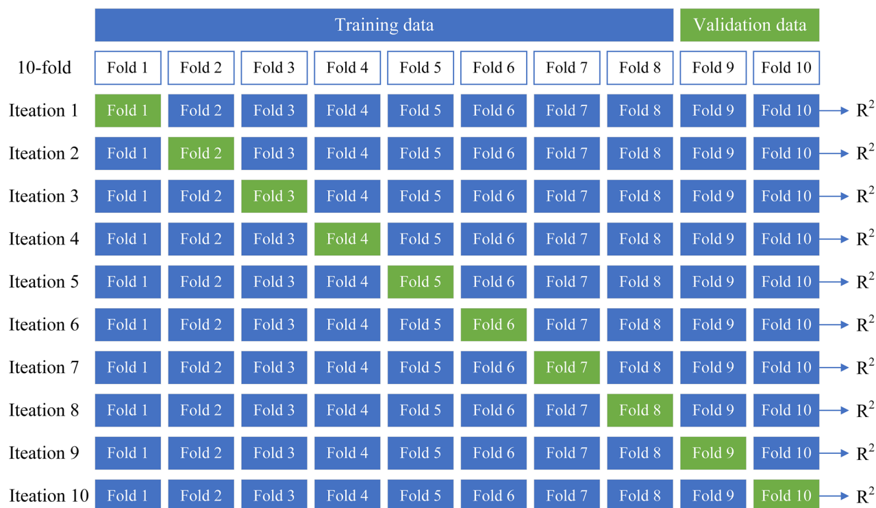
Figure 21. The procedure of tenfold CV.
