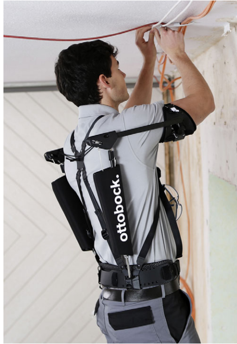
Figure 1. Paexo Shoulder exoskeleton used in construction industry.
