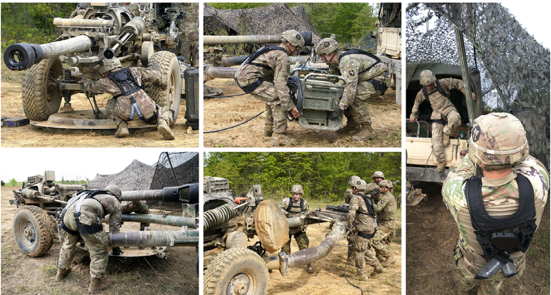
Figure 6. Photos of Soldiers wearing exosuits during a Howitzer emplacement and displacement exercise, as part of an N = 2 case study exploring additional field artillery duties which supplement the formal live fire exercise. Top-left: Soldier reaches under the Howitzer during displacement. Top-middle: Two Soldiers lift and carry a communications box (77 kg). Bottom-left: Soldiers lift a firing platform (102 kg) during Howitzer emplacement. Bottom-middle: Soldiers lift the Howitzer trail end as part of emplacement. Right: One Soldier climbs out of the back of the vehicle while another secures a netting pole.
