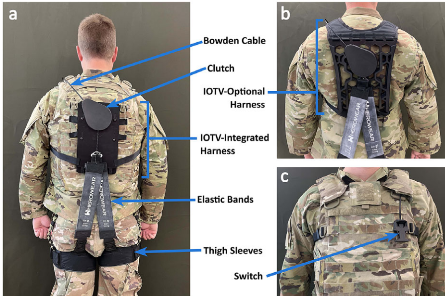
Figure 1. Overview of SABER prototypes. Shown are the (a) back view of the exosuit with the IOTV-Integrated harness, (b) back view with IOTV-Optional Harness, and (c) front view showing the switch. Key exosuit components are labeled. In panel (b), the IOTV is not being worn so that IOTV-Optional harness is visible; however, during field testing, an IOTV was worn over the top.
