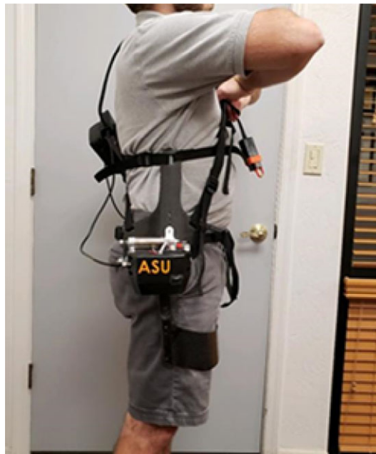
Figure 4. Lumbar plates are used to resist the 30 Nm of torque supplied per motor and keep the back straight during lifting and pushing activities.
