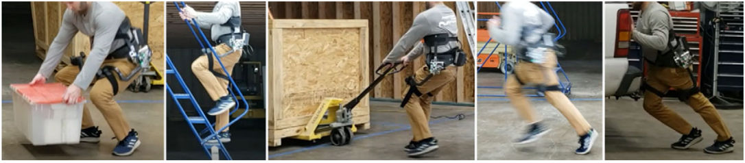
Figure 3. In an active mode, the hip extension is assisted when lifting a box, going up stairs, and pushing a heavy object. During modes such as jogging or running, the block moves out of the way and the hip actuator is in free mode.
