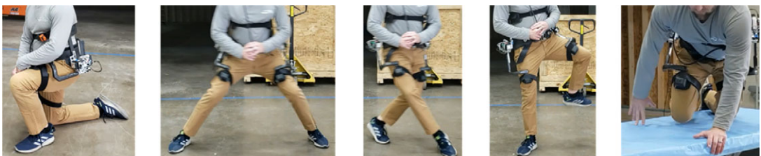
Figure 2. With the motors turned off in a free mode, the user can knee, take wide and cross steps, rotate the hip and crawl.
