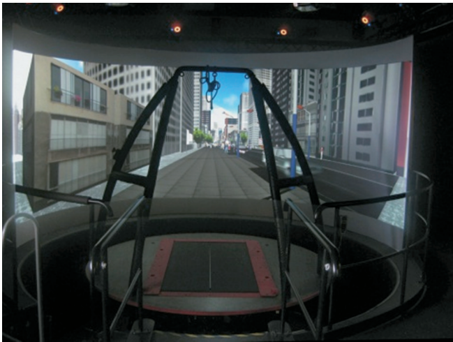
Figure 2.—The CAREN tool consisting of a six-DOF platform, with a dual belt treadmill and a 180° VR screen.
