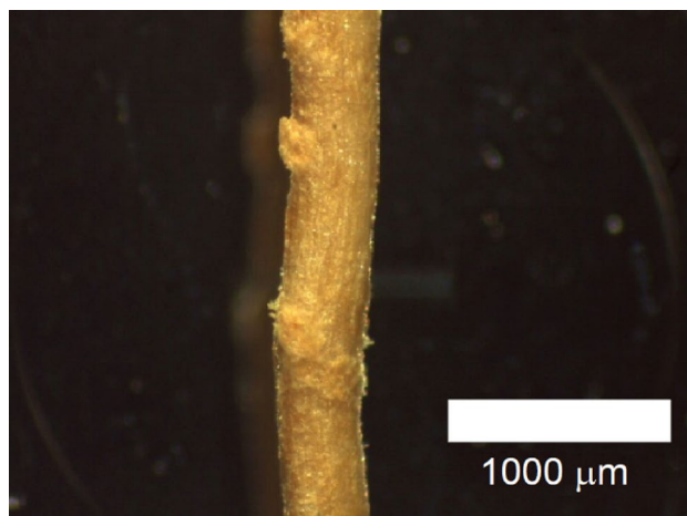
Figure 1. Micrograph of coconut-fiber with the graduated ruler.
