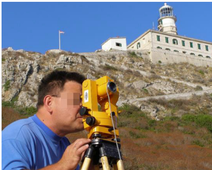
Fig. 3. Observation of the Nord up – ( V_1 ) position during the reoccupation of Palagruža (PALA) RS (a morning set). The DIM instrument is identical to one which is presented in Fig. 2. Applying the tripod, the DIM was installed over the marked RS point.
