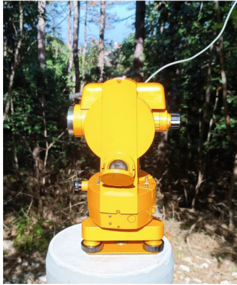
Fig. 2. West up – ( A_2 ) position of DIM device on the outer pillar of Tihany Geomagnetic Observatory. The theodolite is a steal-free Zeiss 020 A equipped with DMI D&I fluxgate probe.
