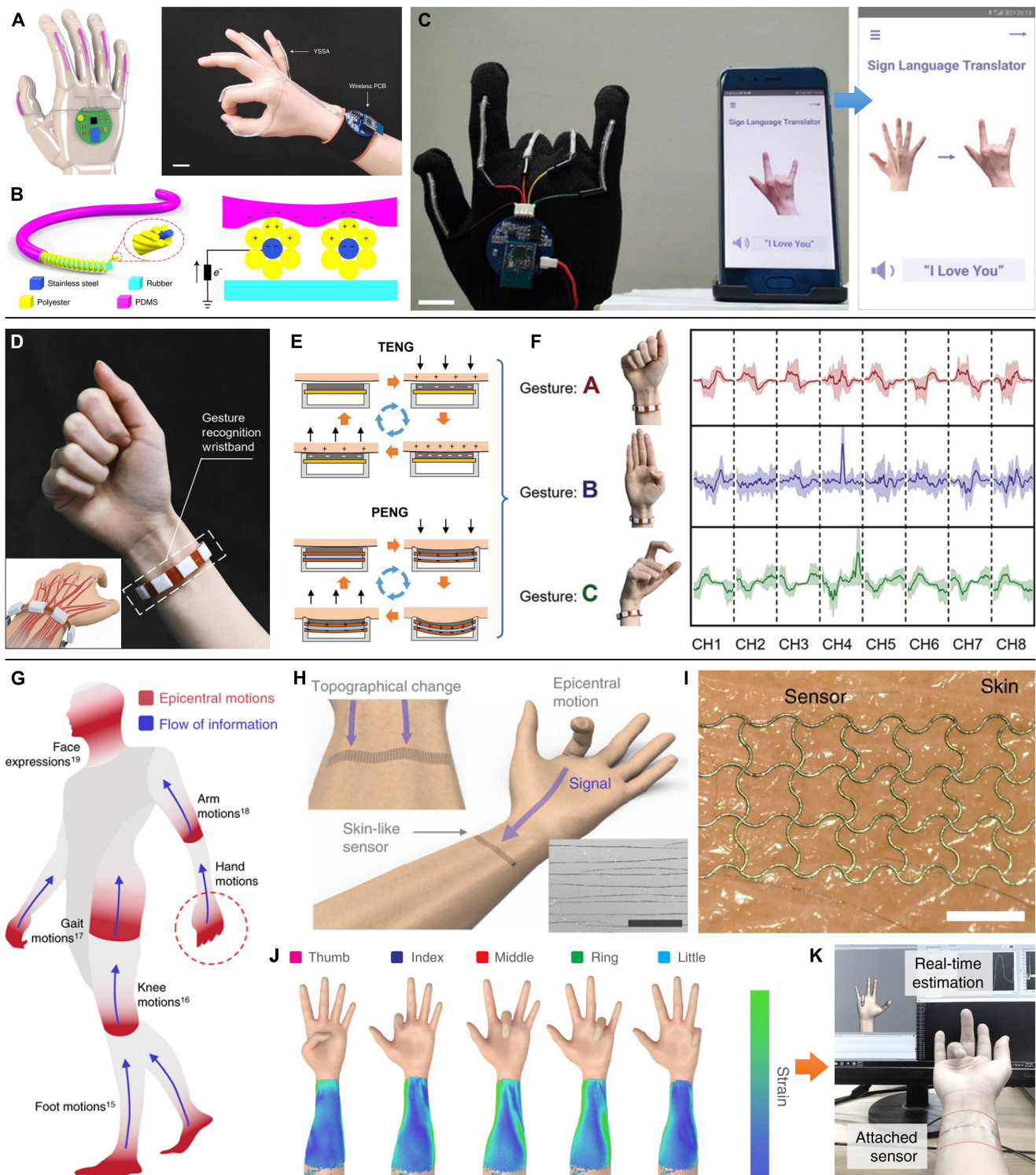
Fig. 5. Tactile sensing devices of gesture recognitions for VR applications. (A to C) Schematic illustration of the triboelectric yarn sensor array (A), working principle (B), and the wearable sign-to-speech translation system (C). Reproduced with permission from [101]. Copyright 2020, Springer Nature. (D to F) Photograph of the gesture recognition wristband sensor (D), working principle (E), and gesture data processing (F). Reproduced with permission from [102]. Copyright 2022, John Wiley and Sons. (G to K) Schematic depicting the possible flow of body information with the epicentral sensor (G), illustration of measuring the epicentral motions of fingers (H) with the insert scanning electron microscopy (SEM) image of the cracked sensor (scale bar, 40 μm), photograph of the sensor conformably on skin (I), depiction of skin deformations for different finger bending motions (J), and photograph of the system for gesture duplication (K). Reproduced with permission from [104]. Copyright 2020, Springer Nature.
