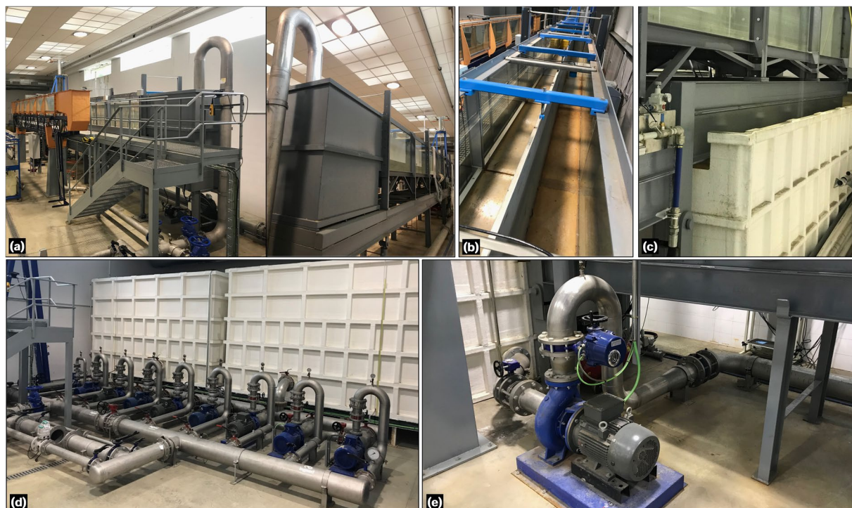
Fig. 1 Photographs of the flume facility: (a) general view, (b) width division wall, (c) cantilever and tailwater reservoir, (d) headwater reservoirs and pumps, and (e) recirculating pump and pipe system.
