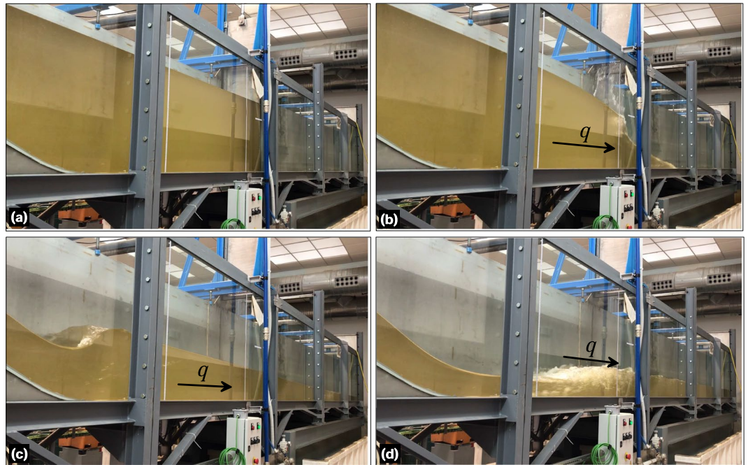
Fig. 5 Photographs of the unsteady hydraulic jump experiment 1 with open tailgate: (a) t = 0 , (b) t \approx 0.5 s, (c) t \approx 3 s, and (d) t \approx 7 s.
