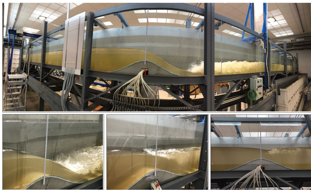
Fig. 4 Photographs of the steady hydraulic jump experiments.
