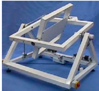
Figure 1. The full-size Random Positioning Machine (RPM); credit Dutch Space. The experiment was fixed in the center of the inner platform during random rotation.
