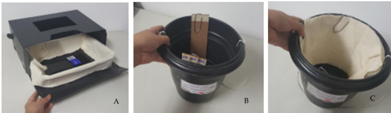
Figure 1. Double BR-ovt oviposition trap (A); Sentinel Ovitrap-OVT-S (B); and control Ovitrap-OVT-C (C). Source: Melo, 2020 [39].
