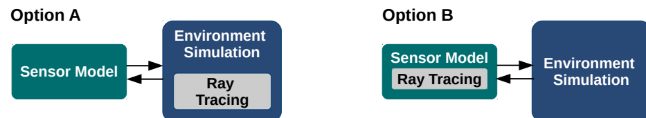
Figure 2. Different options for modular sensor models based on ray tracing. Generally, ray tracing is performed directly in the environment simulation tool (option A). In LiMOX, ray tracing is performed within the sensor model (option B). Due to the internal handling and update of objects, it can even be operated stand-alone.
