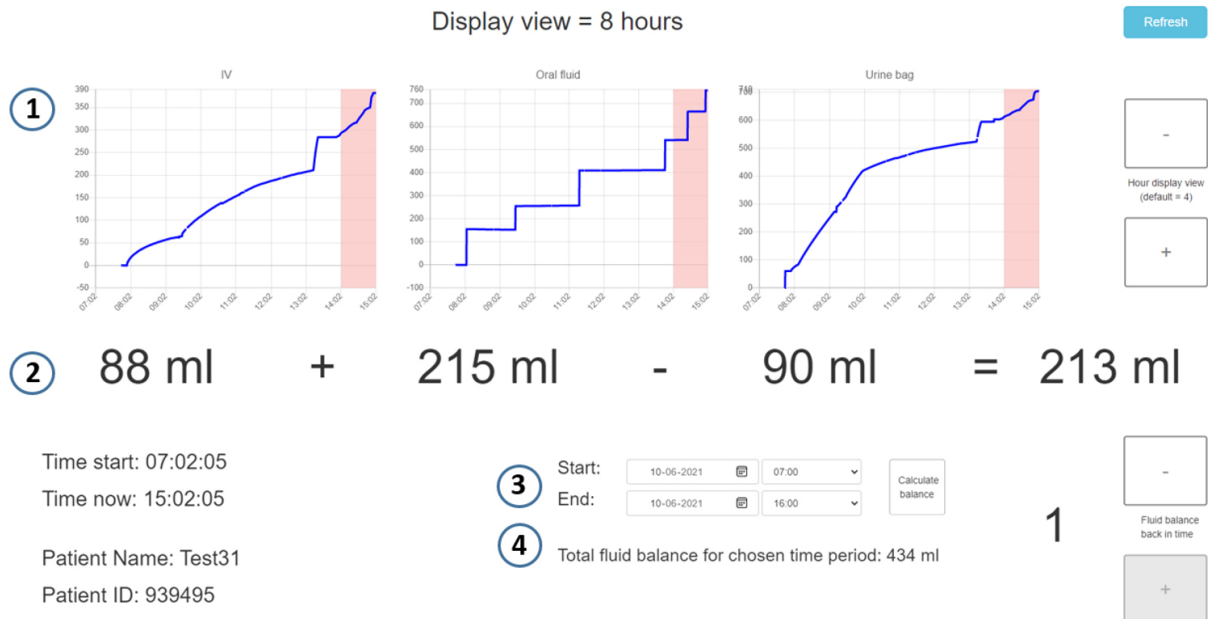
Fig. 2. The graphical user interface displaying data in numbers and graphs. 1) The graphs can display data for up to 10 hours, 2) the large numbers present the volumes of the last hour. 3) Further, you can type in a time period of your choice and 4) LICENSE calculates the total fluid balance for the period.
