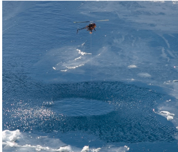
Fig. 2. Profiling operation in areas with significant ice coverage. Note the wire extending from the UAV to the submerged CTD sensor.
