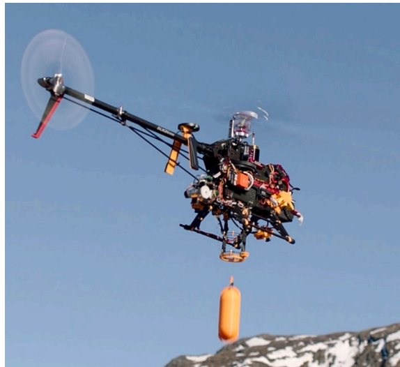
Fig. 1. The complete ARC-AWS UAV with CTD payload (orange) during a test flight. Photo courtesy of Lars Ostenfeld. (For interpretation of the references to colour in this figure legend, the reader is referred to the web version of this article.)
