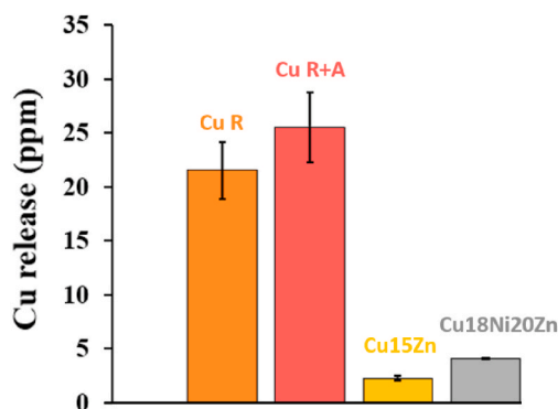
Fig. 10. Cu release amount in artificial sweat (ASW) droplets after 10 min of exposure in quasi-dry conditions.
