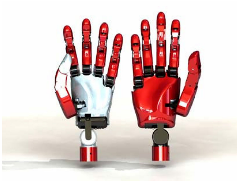
Fig 1: Rendered images of the 50% Female and 50% male 18 DOF Intrinsic hands and 3 DOF Intrinsic Wrists
