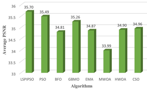
Figure 8. The average PSNR values obtained by different algorithms on all test images.
