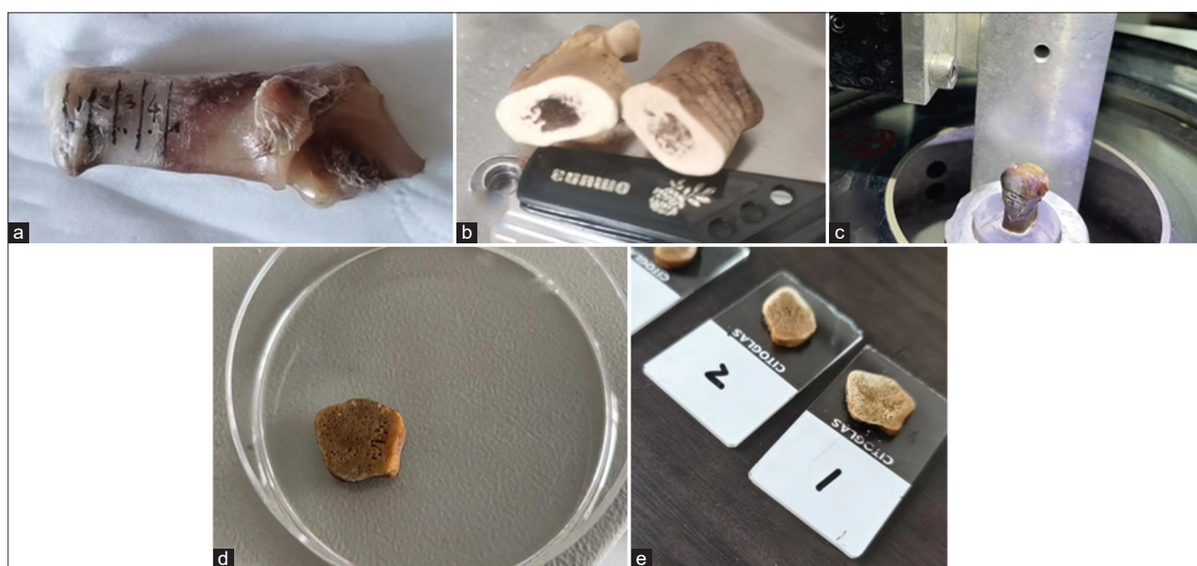
Figure-S2: Serial sectioning and preparation of bone samples. (a) Calcaneus and its regional division, (b) excision of calcaneal diaphysis, (c) fixed the calcaneal diaphysis on the hard tissue microtome (LEICA SP1600), (d) slicing of calcaneal diaphysis, (e) calcaneal diaphyseal cross-section.
