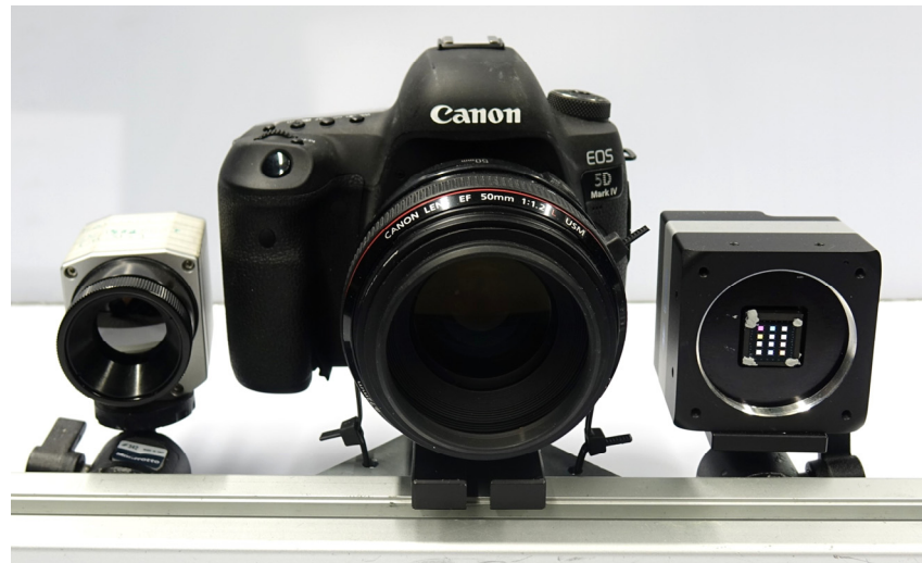
Figure 3. Laboratory setup consisting of a high-resolution DSLR camera ( center ), a 12-channel multispectral camera ( right ), and a thermal camera ( left ).
