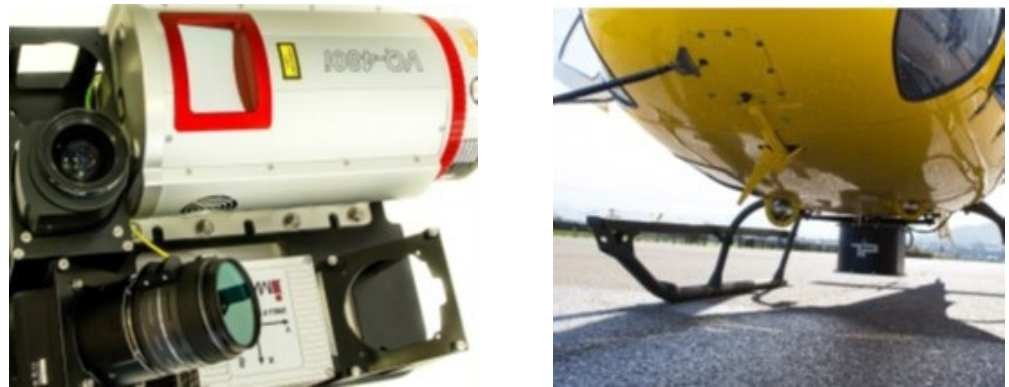
Figure 2. On the left, the laser scanner, two Phase One cameras (zenith and oblique), and the IMU. On the right, the system installed before the flight.
