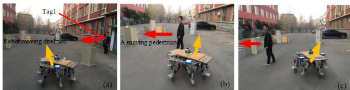
Figure 23. Robot avoids the moving pedestrians. (a) Moves and avoids the obstacles. (b) Encounters a moving pedestrian. (c) Avoids moving pedestrian.
