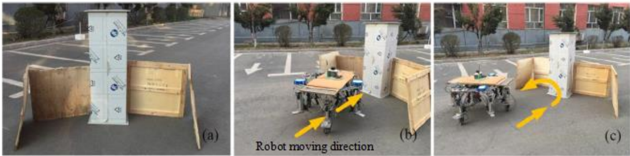
Figure 24. Robot escapes U-shaped trap. (a) U-shaped obstacles. (b) Sinks into U-shaped obstacles. (c) Escapes from the U-shaped obstacle area.
