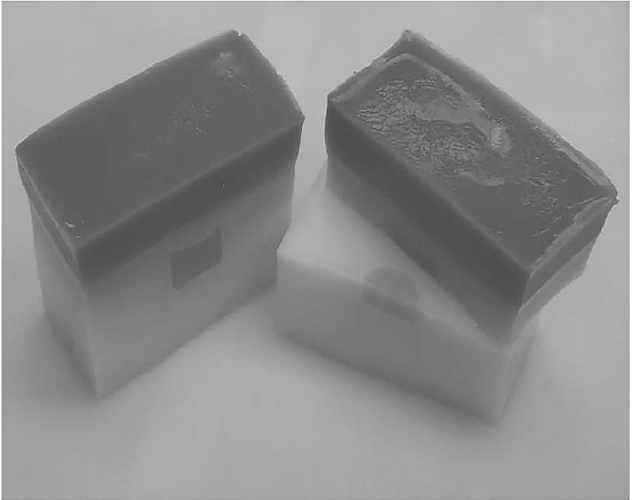
Figure 1. Ultrasound Elasticity Gelatin Phantom
