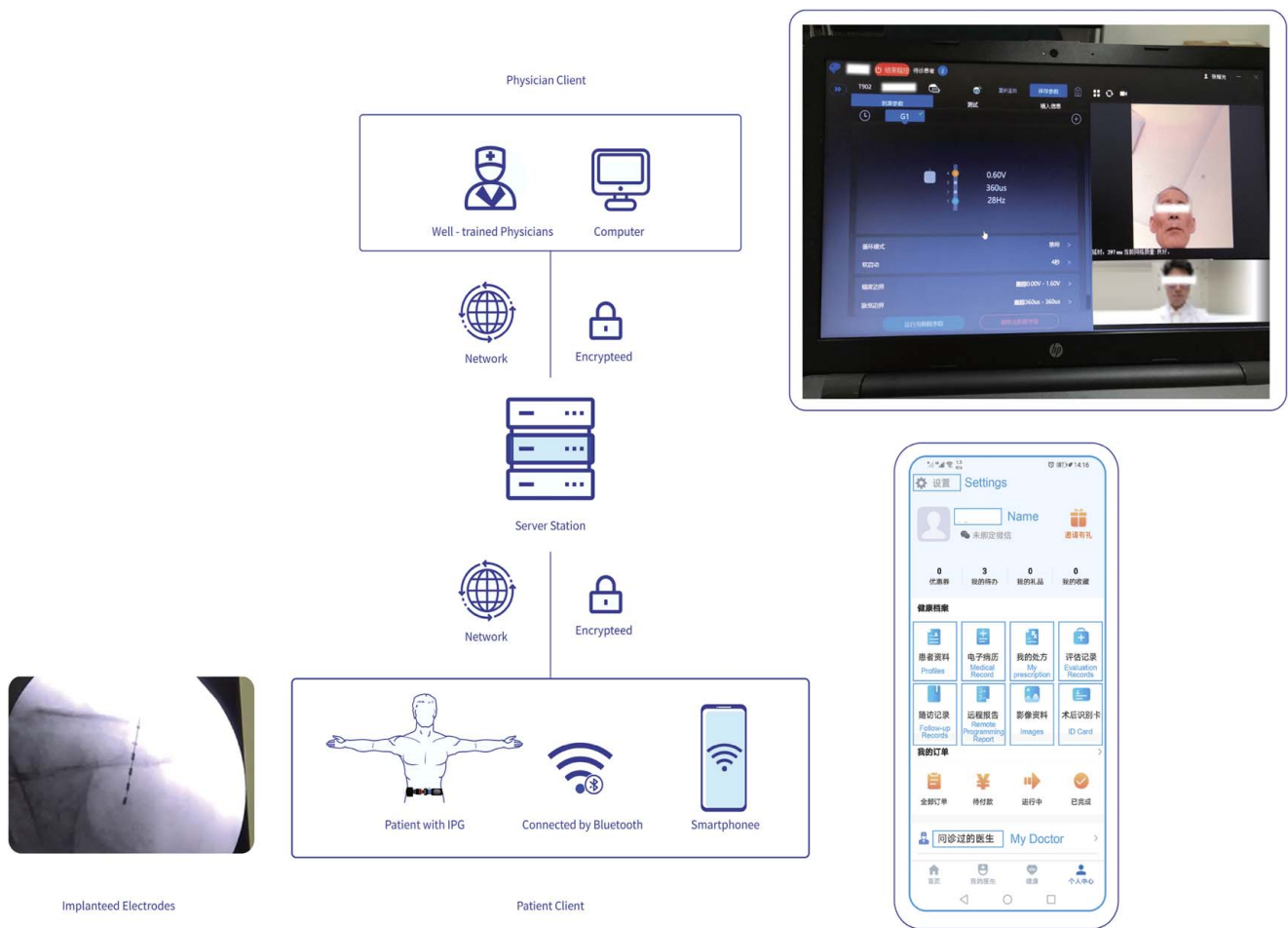
Figure 2. Schematic diagram of how remote programming system works.
