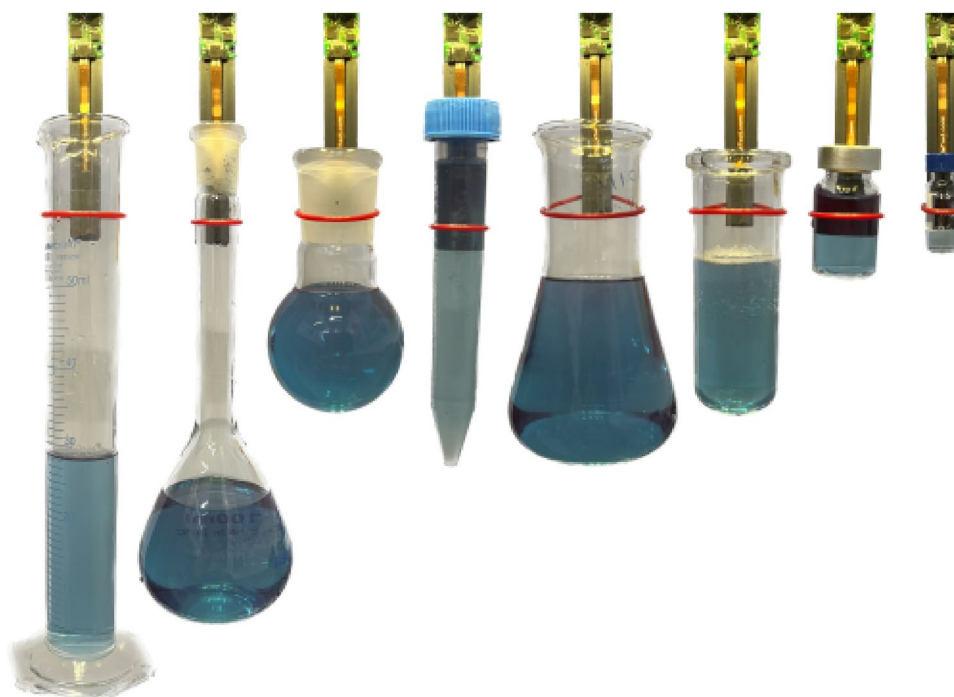
Figure 2. Cable loop gripper prototype grasping various Chemistry glassware.
