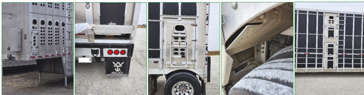
Figure 1. Locations sampled for adenosine triphosphate (ATP) residue using 2 ATP luminometers and bacterial colony-forming units. Trailer locations include from left to right: nose access door (NAD), back door flush gate (BDFG), rear side access door (RSAD), belly flush gate (BFG), and belly side access door (BSAD).
