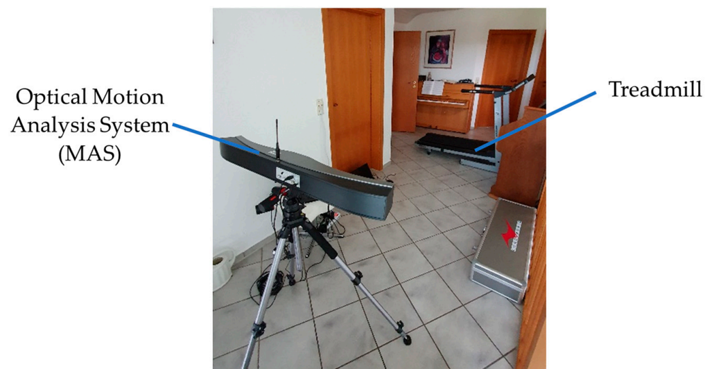
Figure 8. Treadmill test setup with optical MAS positioned 3 m away from the treadmill.
