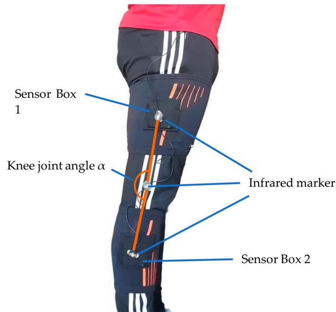
Figure 9. Sensor Boxes attached with bandages to the thigh and shank of the right leg. Additionally, three infrared markers for an optical MAS are attached to the leg. They form a triangle that covers the angle \alpha of the knee joint.
