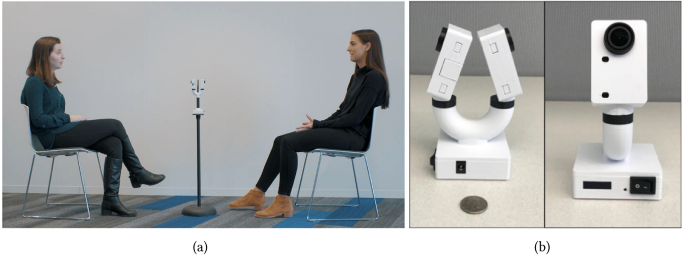
Figure 1: Experimental setup and data collection hardware. In (a), the participant and confederate are having a conversation with the “BioSensor” camera placed between them. In (b), the current model the of “BioSensor.”
