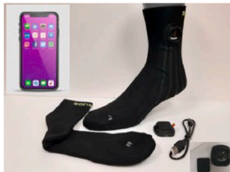
Fig. 2. Example from the sensorised socks in use for the selected use case, where sampling frequency is higher than 50Hz. (Courtesy of Sensoria Inc.).
