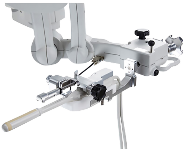
Figure 3. Artemis™ robotic-assisted MRI/TRUS fusion prostate transperineal biopsy platform.
