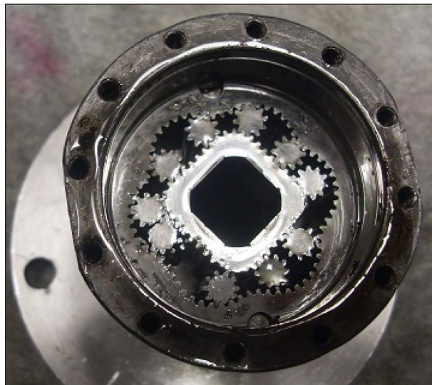
Figure 16. The destroyed satellite mechanism.
