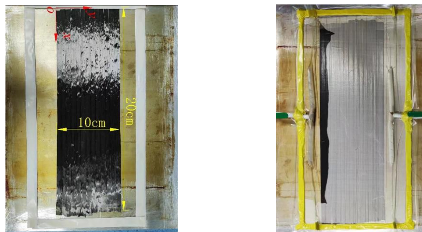
Figure 11. Experiment on measuring the permeability of large-tow carbon fibers.
