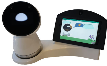
(a) A portable robot station integrated a Jibo robot, Android tablet and Raspberry Pi with a USB camera.
