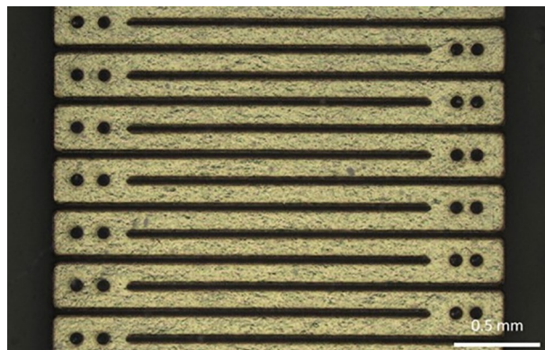
Figure 12. Photograph of one meander-shaped contact of the cuff electrode showing all around the holes made in the contacts to allow anchoring into the silicone sheets.
