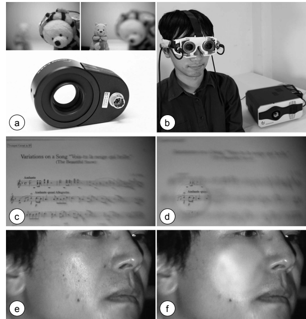
Fig. 6. (Color online) Combining near-eye optics with a high-speed projector enables spatially non-uniformly defocused real-world appearances. 128) (a, b) Two ETLs, capable of quick focus modulation, are used as eyeglasses. (c) The appearance of a music score without the eyeglasses, and (d) with the eyeglasses, where a spatially non-uniform blurring effect guides a player at a fixed tempo. (e) The appearance of a human face without the eyeglasses, and (f) with the eyeglasses, where the facial impression becomes younger by reducing wrinkles and minimizing stains. ( IEEE Trans. Vis. Comput. Graph. 2020, 26 , 2051–2061)
