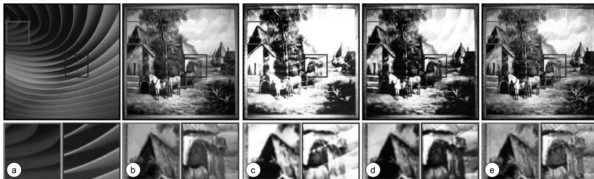
Fig. 2. (Color online) Radiometric compensation using DNNs. 79) (a) Projection target under uniformly white projection. (b) Target appearance. (c) PM result of the target appearance without any compensation. (d) PM result using a classical TPS-based technique. (e) PM result using the DNN-based technique. (2019 IEEE/CVF Conf. Comput. Vis. Pattern Recognit. (CVPR) 2019, 6803–6812)
